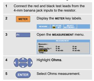
The resistor value is displayed in ohms. Observe also that the bargraph is displayed. (See 15.)
