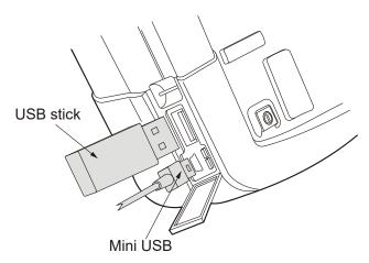
Figure 35. Test Tool USB Connections
