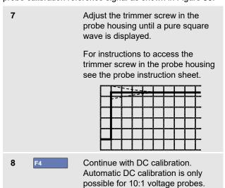
The test tool automatically calibrates itself to the probe. During calibration you should not touch the probe. A message indicates when the DC calibration has completed successfully.
