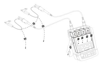
Figure 39. Parasitic capacitance between probes, instrument and environment
