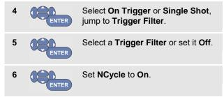
Observe that the key labels at the bottom of the screen have been changed to allow further selection of specific N-Cycle trigger settings:
