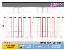
Figure 34. Triggering on Missing Pulses
