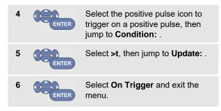
The test tool is now prepared to trigger on pulses that are more than a selectable time in duration. Observe that the trigger menu at the bottom of the screen has been adapted to set the pulse condition:
