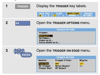
When **Free Run** is selected, the test tool updates the screen even if there are no triggers. A waveform always appears on the screen.
