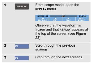
Observe that the bottom of the waveform area displays the replay bar with a screen number and related time stamp:
