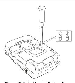
Figure 47. Unlocking the Battery Cover
