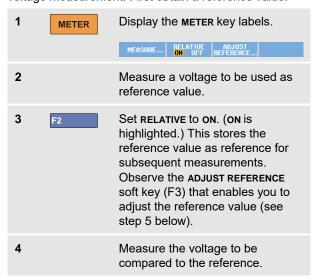
Now the large reading is the actual input value minus the stored reference value. The bargraph indicates the actual input value. The actual input value and the reference value are displayed below the large reading (ACTUAL: xxxx REFERENCE: xxx), see Figure 18.
