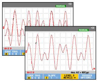
Figure 31. N-Cycle triggering
