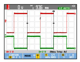
Figure 26. Time Measurement with Cursors
