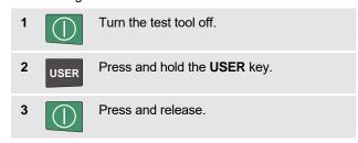
The test tool turns on, and you should hear a double beep, indicating the reset was successful.
