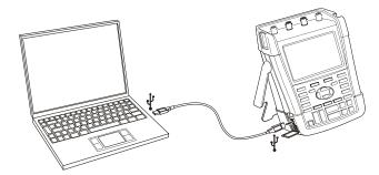
Figure 36. Connecting a Computer
