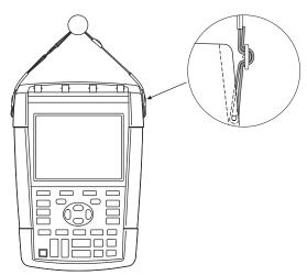
Figure 45. Fixing the Hangstrap
