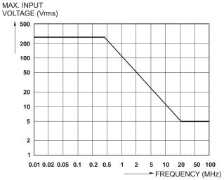
Figure 51. Max. Input Voltage vs. Frequency
