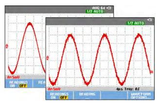
Figure 9. Smoothing a Waveform
