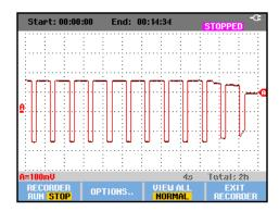
Figure 22. Triggered Single Sweep Recording
