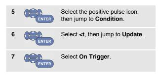
The test tool is now prepared to trigger on narrow pulses only. Observe that the trigger key labels at the bottom of the screen have been adapted to set the pulse conditions:
