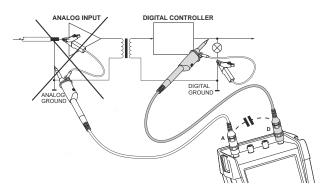
Figure 43. Wrong connection of reference leads
