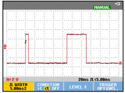
Figure 33. Triggering on Narrow Glitches
