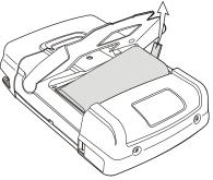
Figure 49. Removing the Battery
