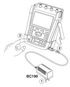
Figure 2. Powering the Test Tool
