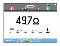
Figure 15. Resistor Value Readings
