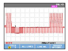
Figure 32. Measuring Interlaced Video Signals
