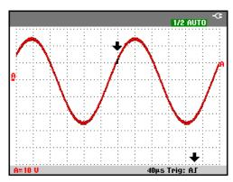
Figure 28. Screen with all Trigger Information
