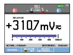
Figure 18. Making a Relative Measurement
