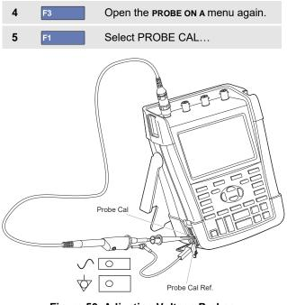
Figure 50. Adjusting Voltage Probes
