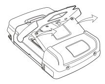
Figure 48. Removing the Battery Cover
