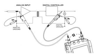
Figure 42. Correct connection of reference leads
