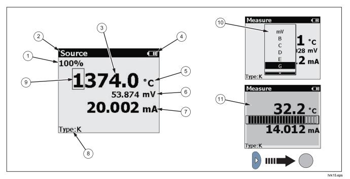
Figure 4. Elements of a Typical Display
