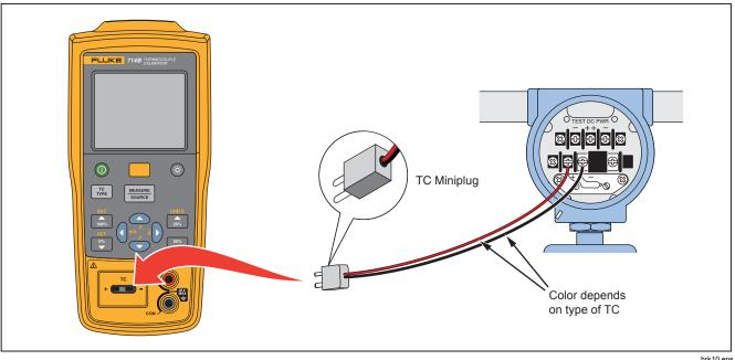
Figure 7. Connections for Simulating a Thermocouple
