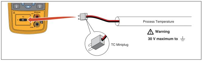
Figure 6. Measure Temperature with a Thermocouple
