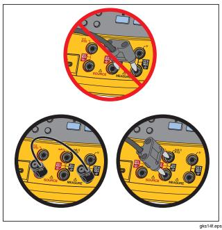
Figure 16. Correct Jumper Use
