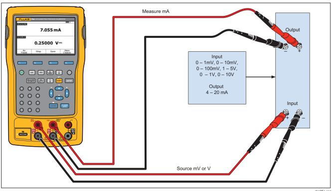
Figure 53. mV to Current Transmitter Calibration
