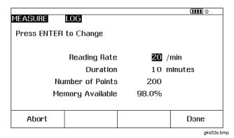
Figure 40. Data Log Parameters Screen
