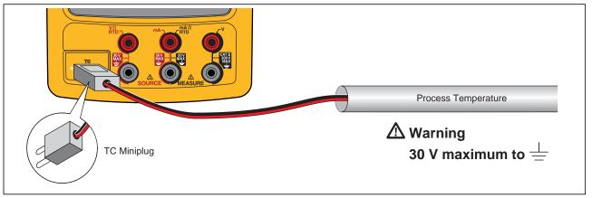
Figure 15. Temperature Measurement with a Thermocouple
