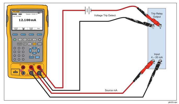
Figure 26. Check a Relay Output Trip Alarm
