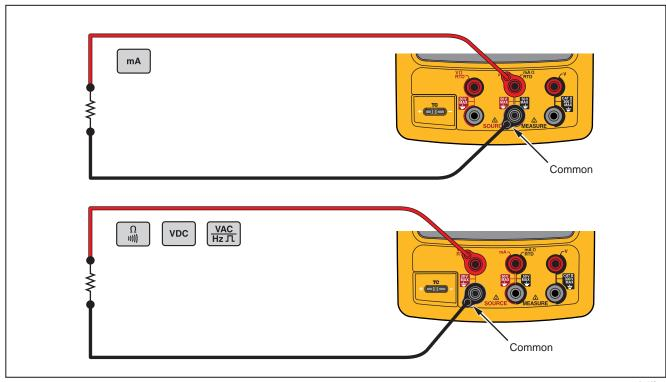
**Figure 18. Electrical Source Connections**
