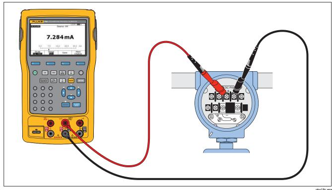
Figure 20. Connections to Supply Loop Power
