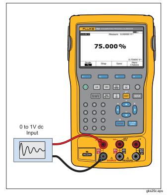
Figure 43. Chart Recorder Calibration
