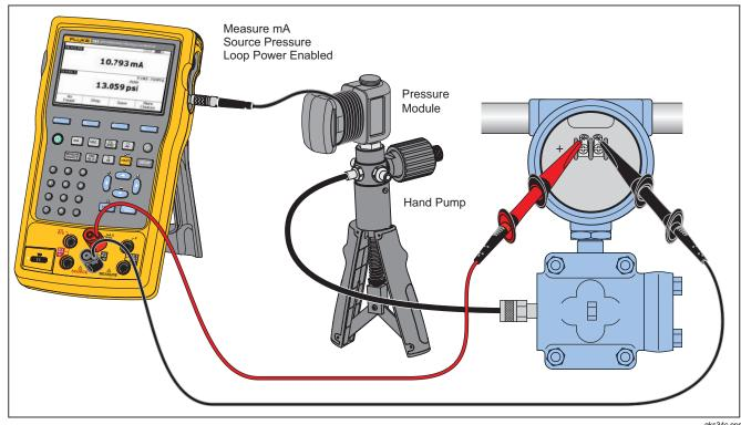
Figure 52. Analog and HART Pressure Transmitter Connection
