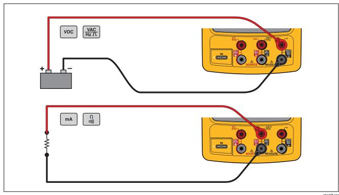
**Figure 12. Electrical Measurement Connections**
