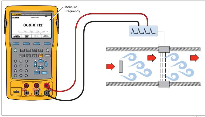
Figure 54. Vortex Shedding Flowmeter Check
