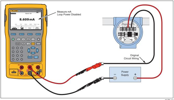
Figure 47. Output Current of a Transmitter Measurement
