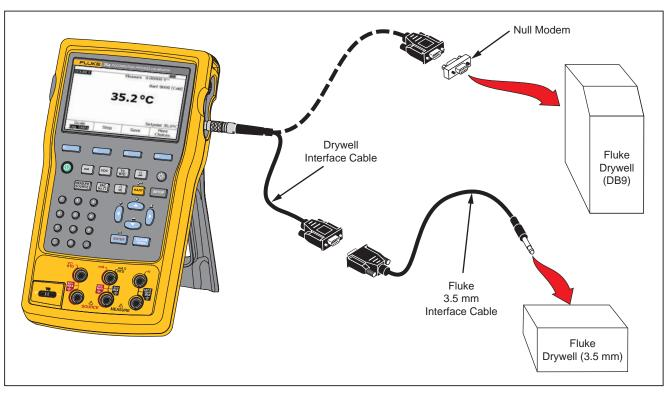
Figure 24. Source Temperature with Drywell
