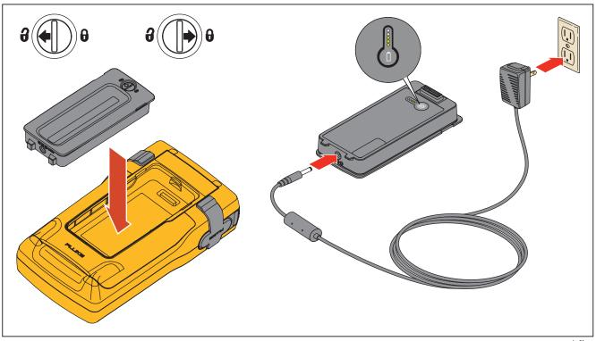
Figure 8. Battery Removal and Charger Use
