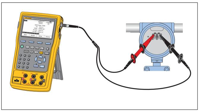
Figure 57. Transmitter HART- Comm Only
