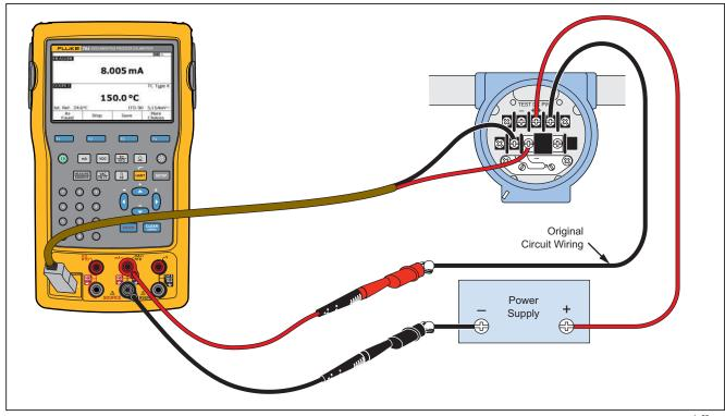
Figure 30. Calibrate a Thermocouple Temperature Transmitter
