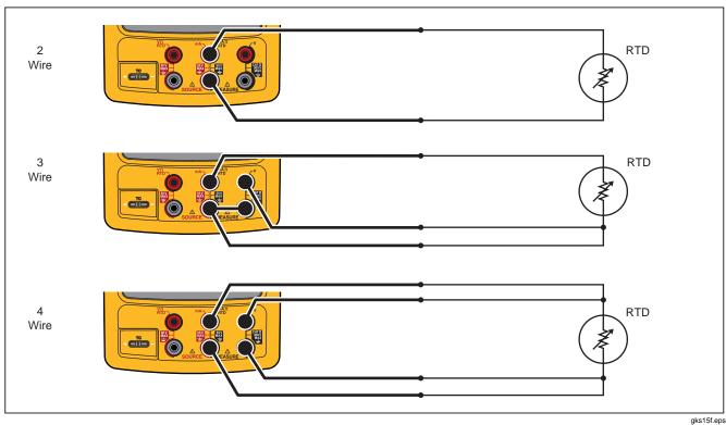
Figure 17. Temperature Measurement with an RTD
