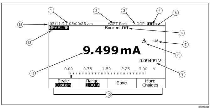
Figure 6. Elements of a Typical Display
