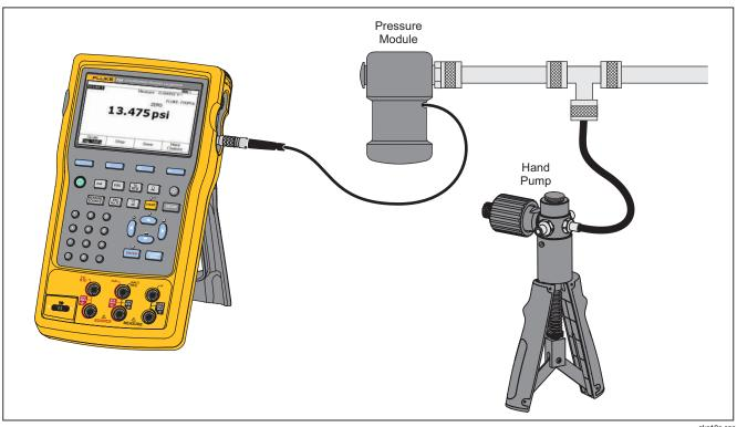
Figure 21. Connections to Source Pressure
