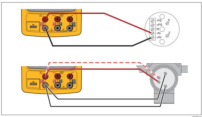
Figure 23. Connections to Simulate an RTD
