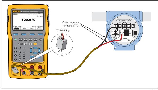
Figure 22. Connections to Simulate a Thermocouple
