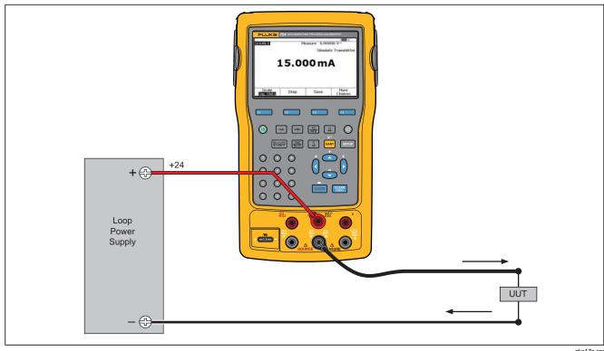
Figure 19. Connections to Simulate a 4 to 20 mA Transmitter
