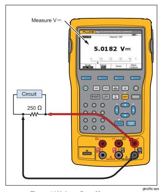
Figure 44.Voltage Drop Measurement
