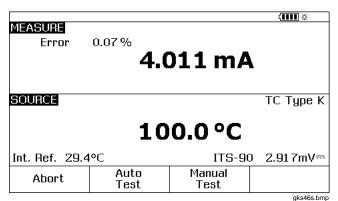
Figure 32. Measure and Source Screen for Calibration
