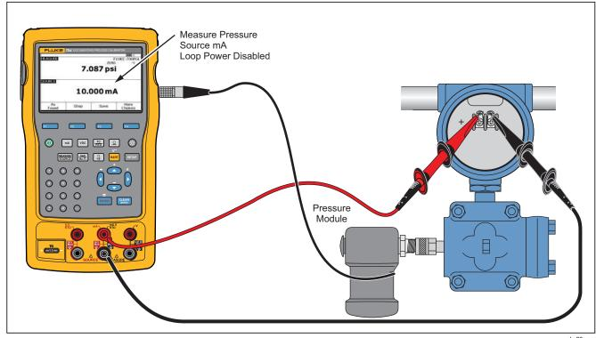
Figure 46. Current-to-Pressure (I/P) Transmitter Calibration
