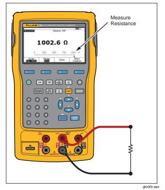
Figure 48. Precision Resistor Measurement
