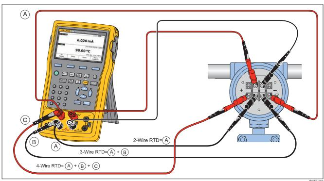
Figure 55. HART and Analog RTD Transmitter Connections
