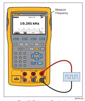
Figure 51. Tachometer Examination
