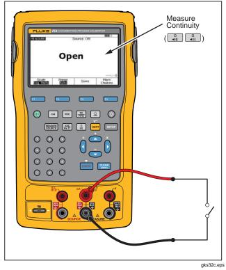
Figure 50. Checking a Switch
