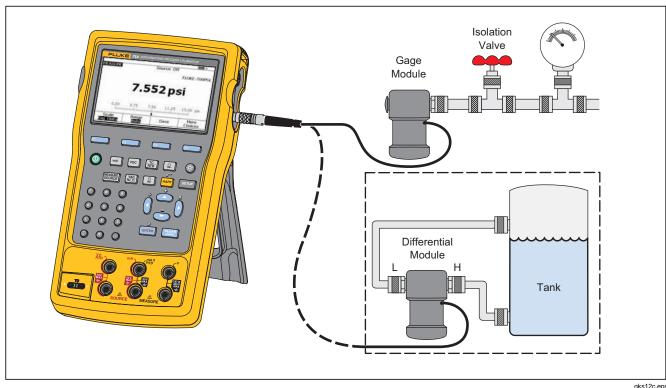
**Figure 14. Pressure Measurement Connections**
