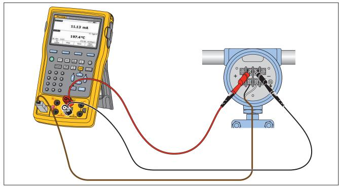
Figure 56. Analog and HART Thermocouple Transmitter Connections
