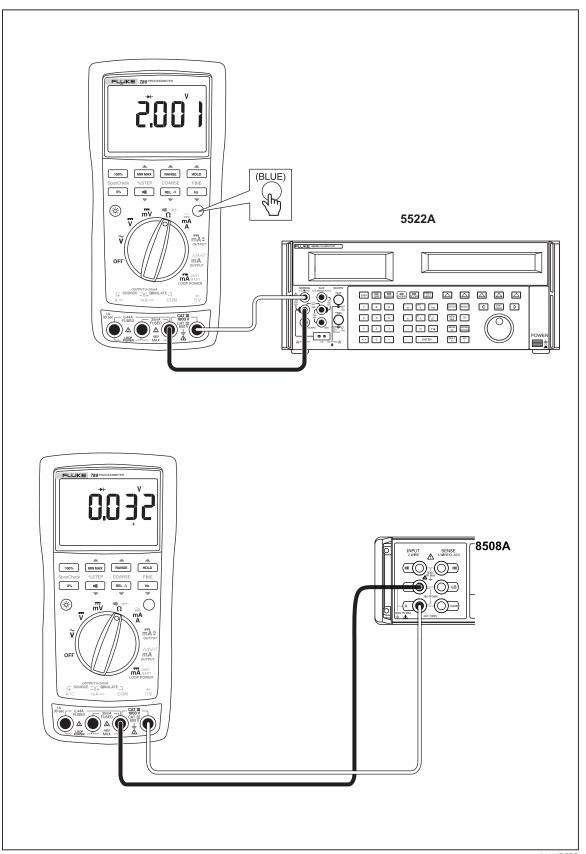
**Figure 5. Diode Test Connections**
