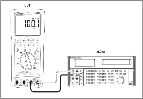
Figure 8. DC mV Measurement Test Connections
