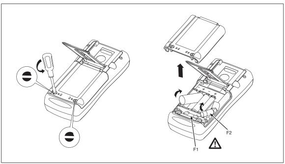
Figure 1. Replacing the Batteries and Fuses
