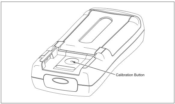
Figure 11. Calibration Button Access
