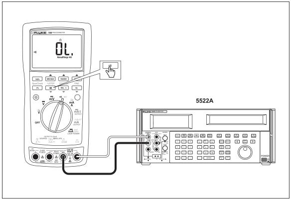
**Figure 6. Continuity Test Connections**
