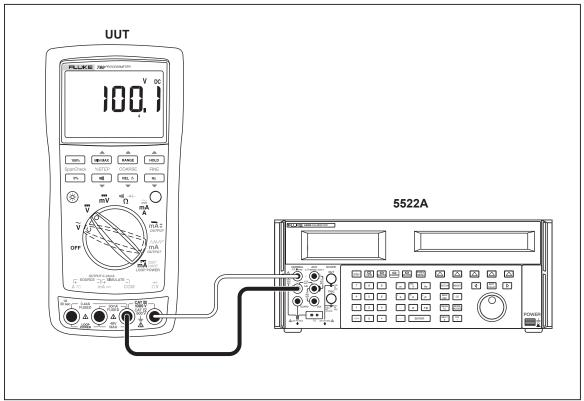
Figure 9. AC/DC Voltage Measurement Test Connections
