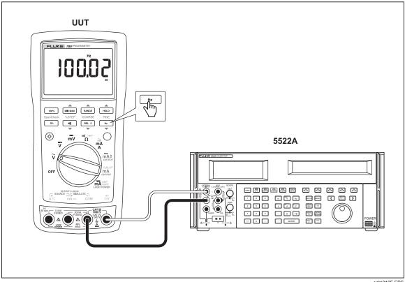
Figure 10. Frequency Measurement Test Connections
