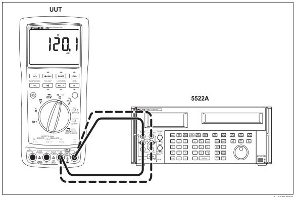
Figure 7. Resistance Measurement Test Connections
