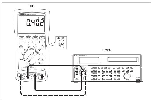
**Figure 4. Current Measurement Test Connections**
