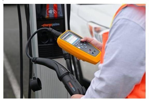
The solution includes TruTest™ EV Charging software module for documentation and reporting. The solution performs these measurements: PE (protective) earth pre-test, visual inspection, GFCI trip test, nominal voltage, auto control pilot (CP) with waveform analysis, proximity pilot, and error testing. Seamless integration with TruTuest software via Bluetooth connection for simplified report generation.
