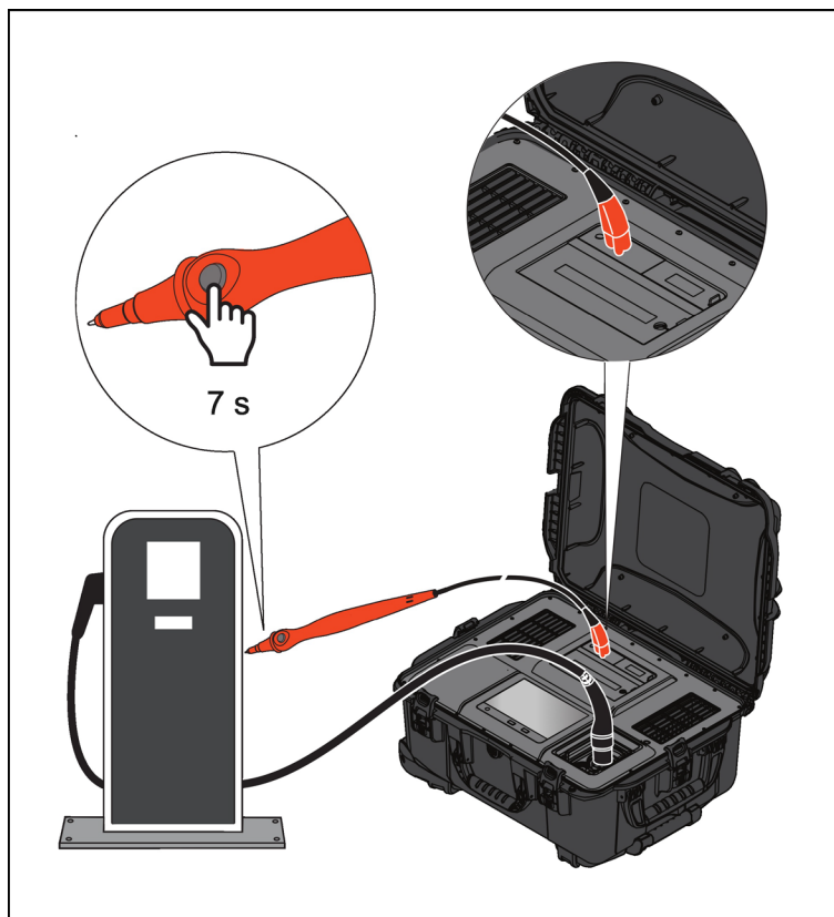
Figure 5. Performing Continuity Test
