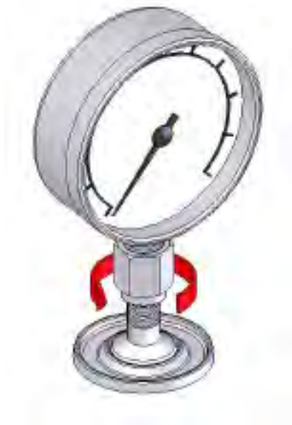
Figure 2-2. Connect Assembly to Test Port
