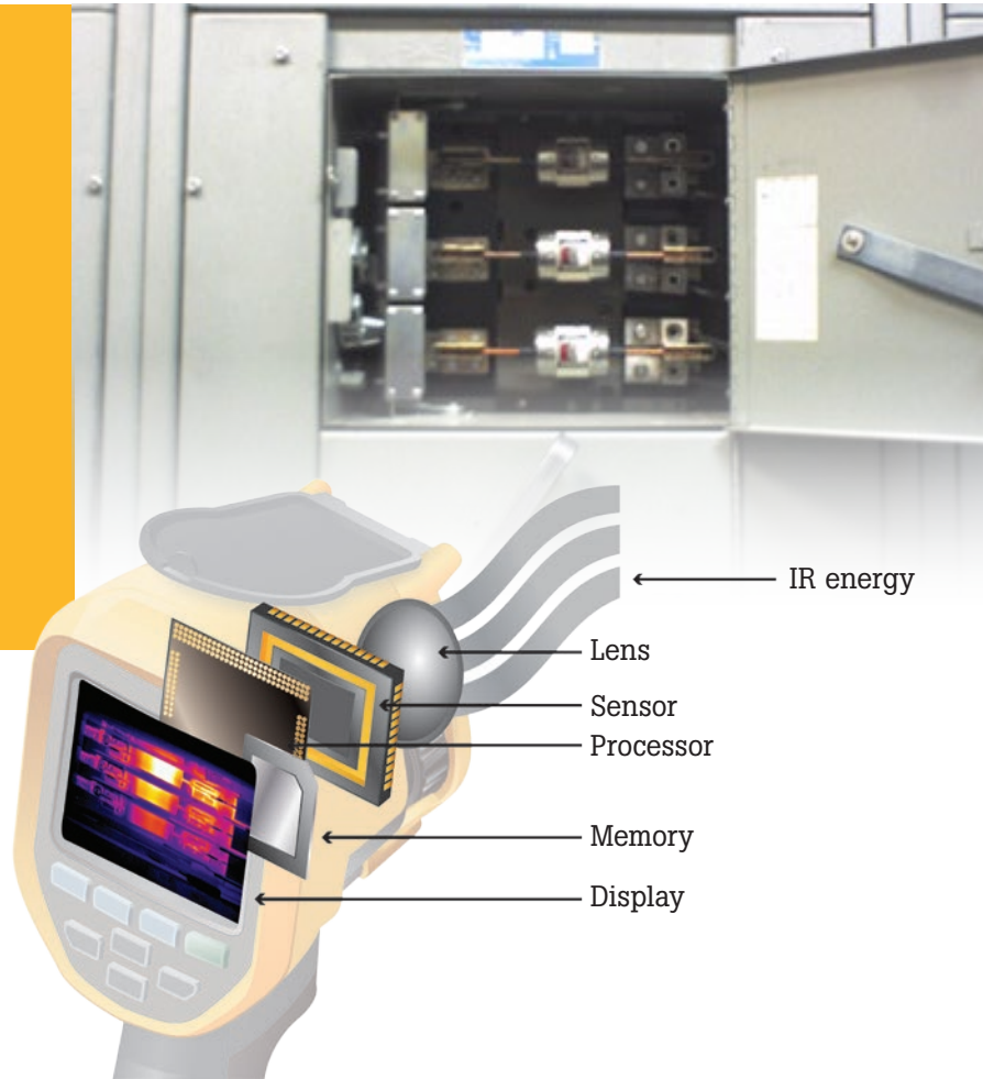
Figure 1. Anatomy of an infrared camera
